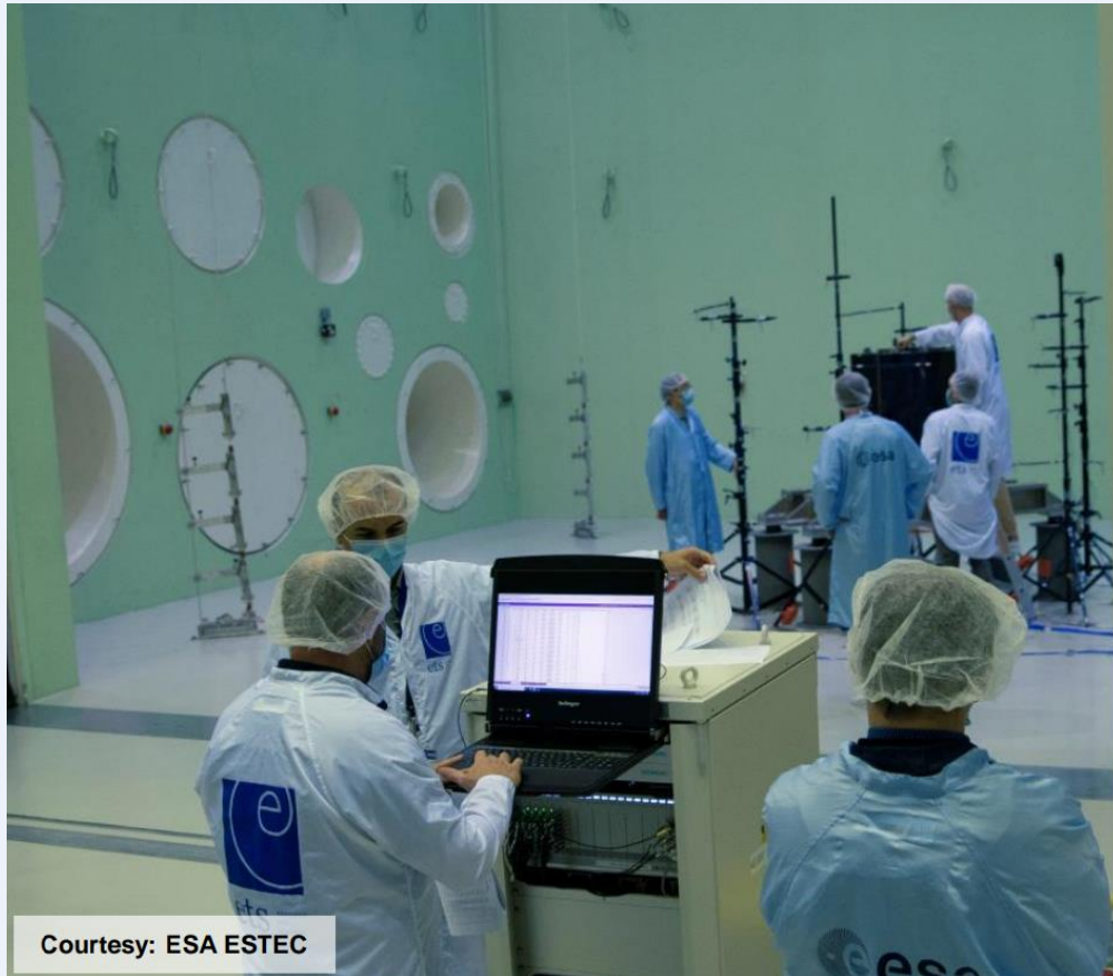
Reverberant field acoustic noise testing
