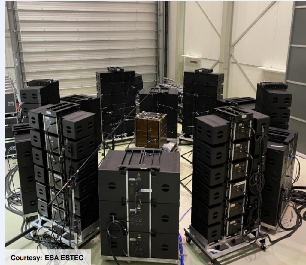
Direct field acoustic noise testing
