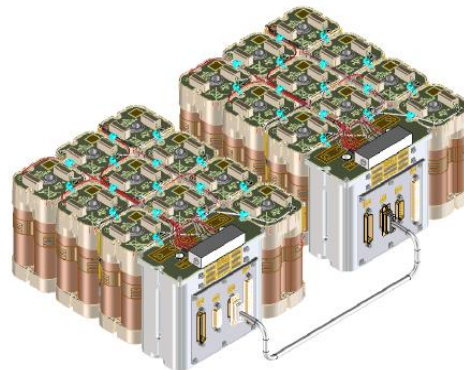
Copernicus CIMR Battery Configuration (8S5P)2S
